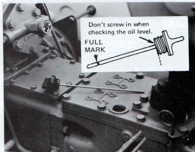
Figure 39 — Transmission, Rear Axle and Hydraulic System Oil Level Dipstick and Fill Plug
