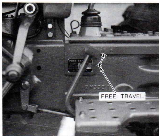
Figure 61 — Clutch Pedal Free Travel Adjustment
